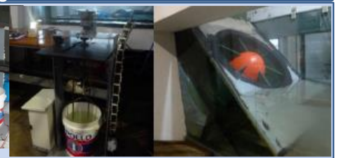
Fig. 9 Installation testing of axial turbine with PMG system
