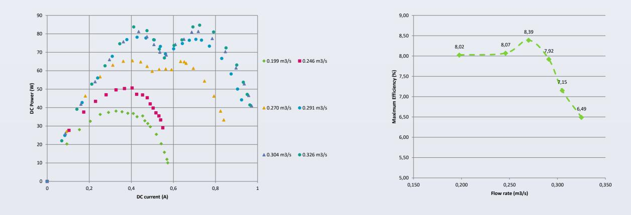
Shown that at every flow rate has maximum DC power also. At flow rate 0.270m<sup>3</sup>/s, 0.291m<sup>3</sup>/s, 0.304m<sup>3</sup>/s, and 0.326 m<sup>3</sup>/s, the power has two peaks due to STAVOLT activity. From Fig 4.b known that the highest efficiency of DC system was 8.39% obtained at flow rate 0.270m<sup>3</sup>/s with efficiency of ATPMG 9.3%, STAVOLT efficiency 97.35% and Rectifier efficiency 92.72%.
